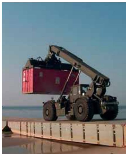
KALMAR RT240 RTCH unloading vessels via pontoons
