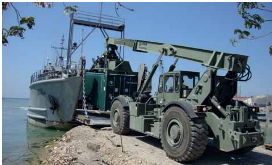
KALMAR RT240 RTCH unloading landing vessel
